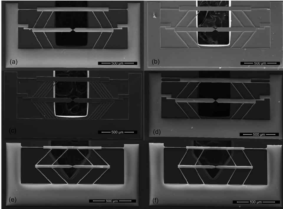
Fig. 1. SEM images showing variations of the microdevice; devices labeled (a)–(d) belong to generation I, while devices labeled (e) and (f) belong to generation II. The devices labeled (a) and (f) are composed of inclined beams making a  $60^\circ$  angle with the sample-stage shuttles. The rest of the devices have inclined beams making a  $45^\circ$  angle with respect to the sample-stage shuttles.
