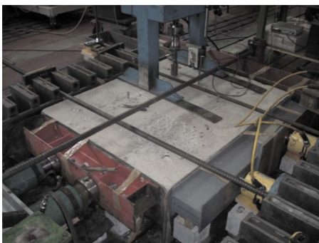
Fig. 5. Detail of the built-in frame with the testing machine
