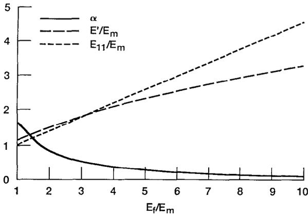
FIG. 11. Nondimensional parameters  $\alpha$ ,  $E'/E_m$  and  $E_{11}/E_m$  vs  $E_f/E_m$  for composite with  $v_f = 0.3$ ,  $v_m = 0.35$  and  $f = 0.4$ .
