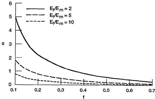
FIG. 10. Nondimensional parameter  $\alpha$  vs fiber volume fraction  $f$  for several composites with  $\nu_f = 0.3$  and  $\nu_m = 0.35$ .
