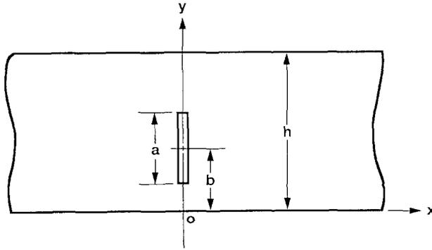
FIG. 1. Configuration of the cracked strip.
