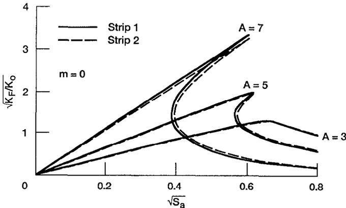
FIG. 8. Normalized shielding stress intensity factor vs normalized loading parameter for bridged edge crack under uniform tension.
