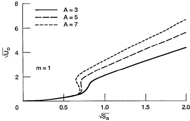
FIG. 3. Normalized crack mouth opening displacement vs normalized loading parameter for bridged Griffith crack.
