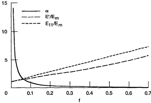
FIG. 9. Nondimensional parameters  $\alpha$ ,  $E'/E_m$  and  $E_{11}/E_m$  vs fiber volume fraction  $f$  for composite with  $E_f/E_m = 10$ ,  $\nu_f = 0.3$  and  $\nu_m = 0.35$ .
