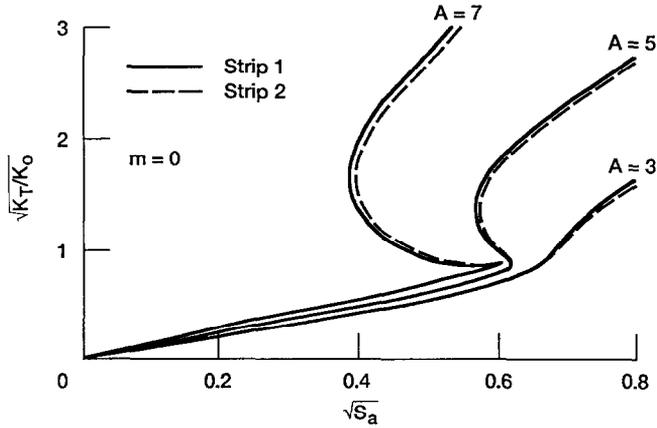
FIG. 7. Normalized total stress intensity factor vs normalized loading parameter for bridged edge crack under uniform tension.
