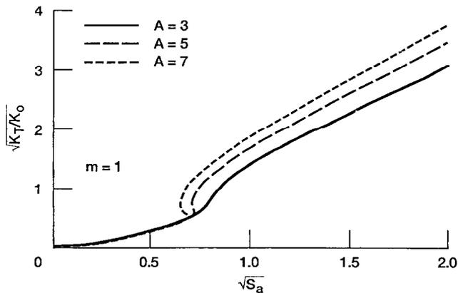
FIG. 4. Normalized total stress intensity factor vs normalized loading parameter for bridged Griffith crack.
