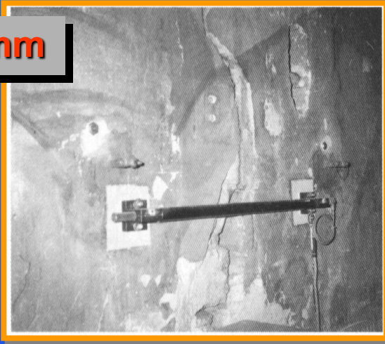
View of a 70 cm displacement transducer
