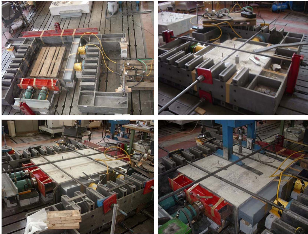
Fig. 5. Built-in frame for the application of compressive prestress using hydraulic jacks
