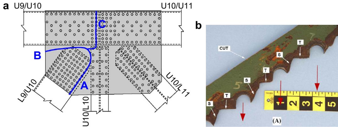
**Fig. 3.** (a) Node U10 of I-35W Bridge showing gusset plate connecting truss members. The blue lines labeled A, B, C represent the observed cracking patterns within the gusset plates. A and C indicate cracks that linked the rivet holes. (b) Part of the gusset plate indicating the ductile tearing of the ligaments between the rivet holes; S and T represent shear and tension, respectively (Refs. [8,9]).
