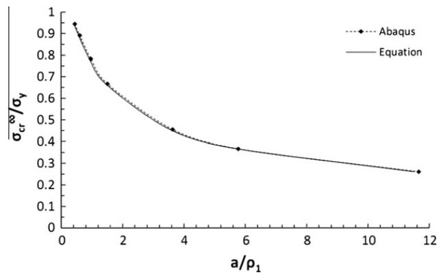
Fig. 2. Normalized strength versus structural size/brittleness predicted by Dugdale model.
