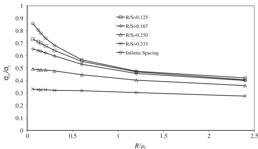
Fig. 6. Nominal strength of plate with periodic arrangement of holes as functions of brittleness.
