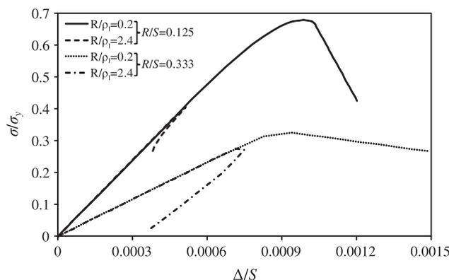
Fig. 7. Nominal stress–nominal strain curves of plate with periodic arrangement of holes for selected values of spacing and brittleness number.
