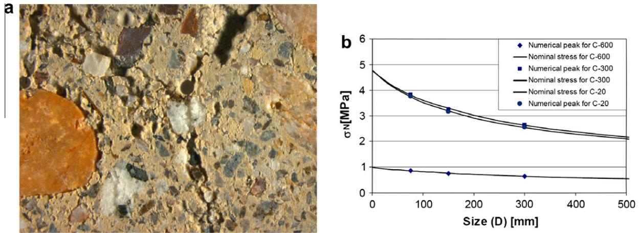
**Fig. 4.** (a) Micrograph of concrete microstructure after exposure to 600 °C. (b) Normalized strength of concrete at 20 °C, 300 °C and 600 °C as functions of specimen dimensions. (Ref. [10]).
