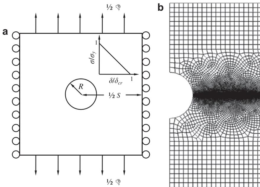
**Fig. 5.** (a) Micromechanics model. (b) Finite element discretization of micromechanics model.
